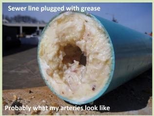
Just like a human artery, when a sewer line becomes constricted it does not function properly. Over time the constriction becomes worse until the line may become completely blocked. For a human that would lead to a heart attack.
