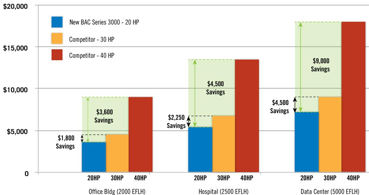
Energy Cost Savings Based on a 400-Ton System (\$0.12 kWh)
